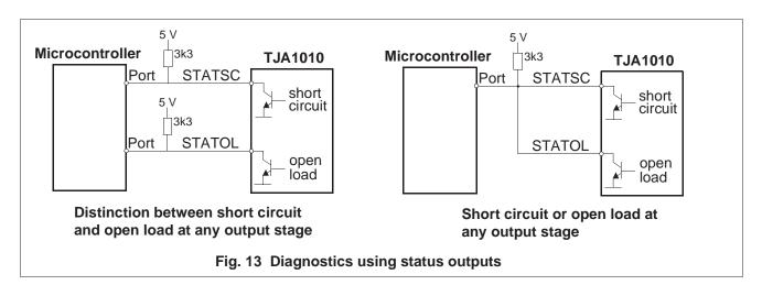
Channel selective diagnostic information can be derived by evaluating the serial output data of the TJA1010 with the microcontroller. For this purpose, the actual data received from the TJA1010 (new bits) have to be compared with those previously sent to the TJA1010 (old bits). Table 7 shows, that a fault detection at a certain output stage is indicated, if the old and new bit at the respective position are unequal. Otherwise, no fault has been detected.
