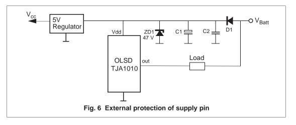
Table 5 summarizes the TJA1010 behaviour with the protection circuit in figure 6, when applying the most commonly required test pulses for a 12 V vehicle supply system.
