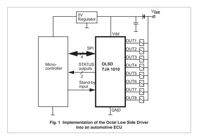
The intention of this Application Note - together with the data sheet of the device [1] - is to provide the information, which the designer needs for a successful implementation of the TJA1010 into his ECU.
