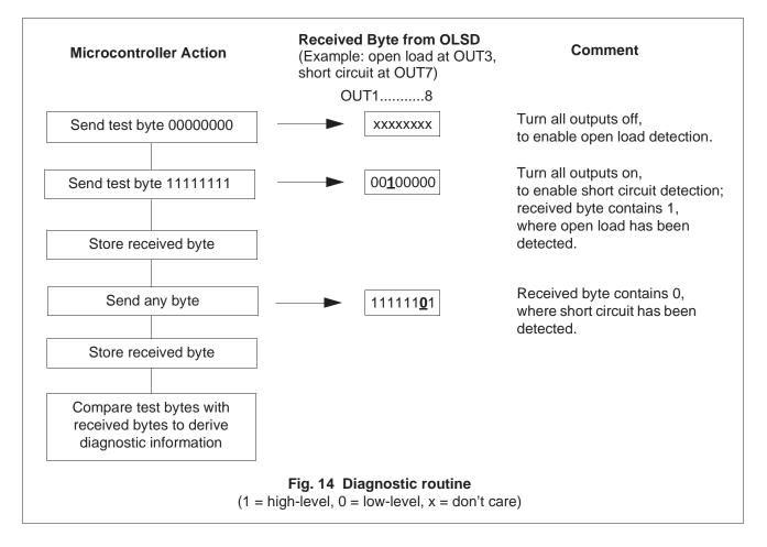
If any short circuit condition has been detected, the respective output stages or - in case of emergency temperature shutdown - all output stages should be turned off until the failure has been removed. Otherwise, the operation of the device at one of the two temperature protection levels over a long time would reduce its reliability.
